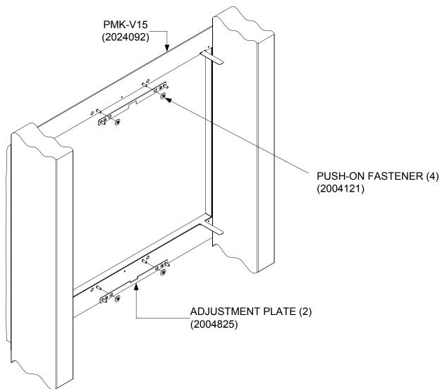
2. Slide a push-on fastener over each pin of the PMK-V15 (or BB-V15) to loosely secure the adjustment plate and the mounting plate. Do not push the push-on fasteners all the way down onto the pins. Slide them on enough to keep the adjustment plate and mounting plate as one adjustment/mounting plate assembly.
