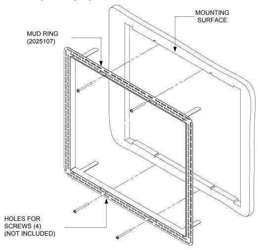
**NOTE**: SCREW LENGTH SHOULD NOT EXCEED MOUNTING SURFACE THICKNESS BY MORE THAN 1/2" (13 MM).
