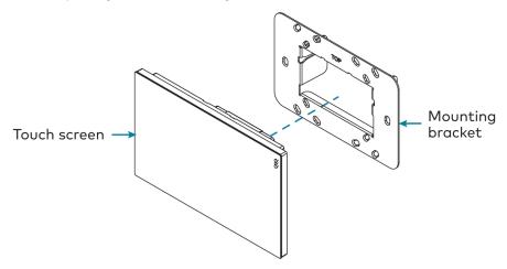
If the touch screen is not level after installation, pull it out of the mounting bracket and loosen the screws holding the bracket into place. This procedure allows the mounting bracket to be rotated slightly.
