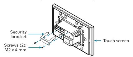
To remove the touch screen after installation, use the included release key to push down on the security bracket release tabs as shown in the following illustration while gently pulling the touch screen away from the mounting bracket.
