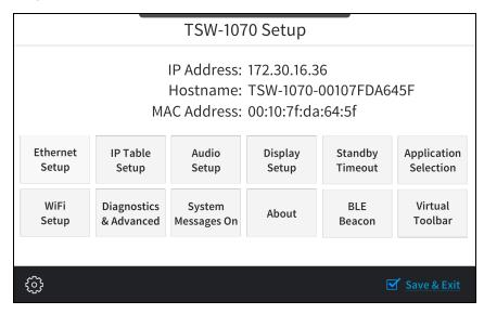
Use the setup screens to configure various settings for the touch screen, including Ethernet setup, IP table setup, audio setup, display setup, standby timeout, Wi-Fi network setup, and diagnostics.
