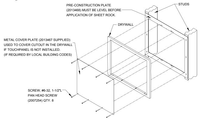
**NOTE:** Prior to mounting the touchpanel, ensure that the PMK-17L is flush with the drywall (no kinks or bends in the metal). Any separation may make screwing in the touchpanel more difficult. One can purchase and attach a TMK-17L or MMK-17L to keep the PMK-17L straight.
