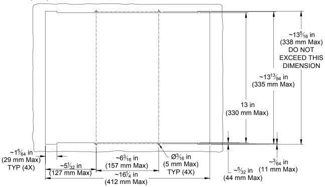
If the opening for the touchpanel in the drywall is too large, two pre-construction accessories are available to make adjustments. Use the optional TMK-17L (Trim Ring Kit) to provide a smooth edge at the opening. This option provides a finished appearance and is preferred when wallpaper is hung. Use the optional MMK-17L (Mud Ring Kit) to fill in larger irregularities around the opening (requires plastering).
