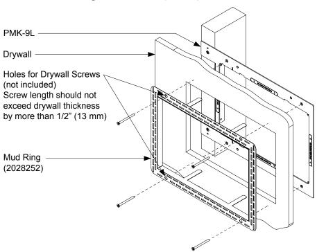
Insert and Secure Mud Ring Plate into PMK-9L (or BB-9L)
