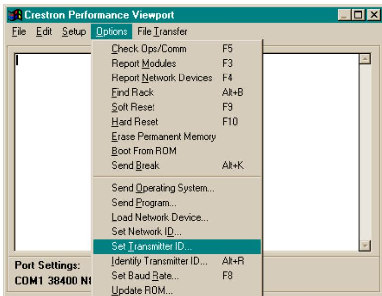
From the Options menu in the dialog box, select Set Transmitter ID to open the “Set Transmitter ID” dialog box. Enter a two-digit hexadecimal number ranging from 03 to FE. Click OK to confirm.
