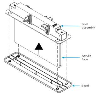
4. Slide the bezel retained during the disassembly carefully over the acrylic face until the magnets on the bezel snap into place against the SSC assembly.
