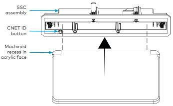
1. Align the replacement acrylic face with the SSC assembly so that the side of the face with the machined recesses is facing away from the side of the assembly with the CNET ID button.
