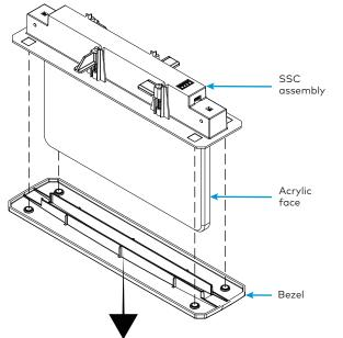
1. Remove the bezel from the SSC assembly by gently pulling it away from the installed sign to break the magnetic hold, then sliding it down and across the acrylic face. Retain the bezel.
