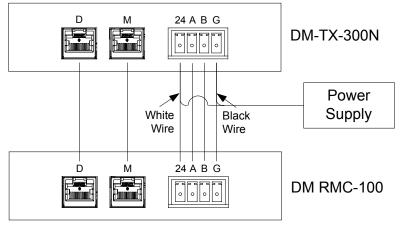
**NOTE:** When using a single supply, ensure it provides sufficient power for both devices.
