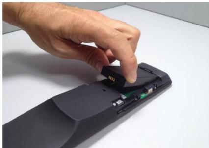
4. Reattach the battery compartment cover by pressing down lightly on the locking tab while sliding the cover into place.
