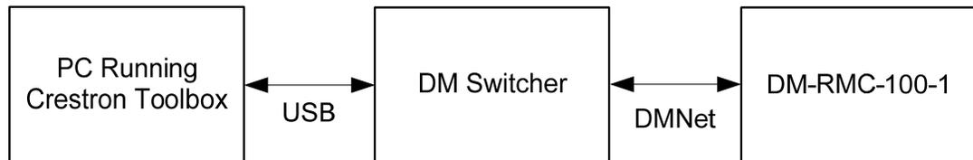
To establish USB communication between the PC and the DM-RMC-100-1 via a DM switcher:
