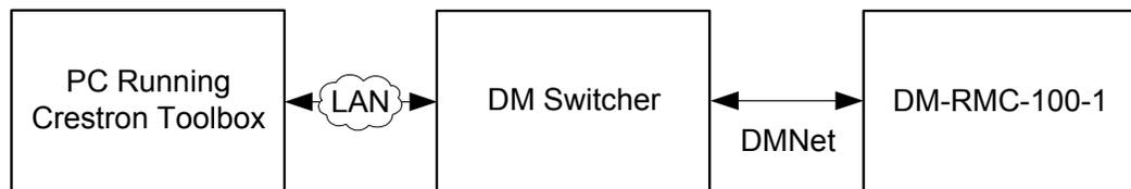
To establish TCP/IP communication between the PC and the DM-RMC-100-1 via a DM switcher:
