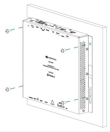
**NOTE:** The anchors are best suited for surfaces with 3/8 in. to 3/4 in. thickness.
