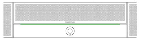
• Muting the microphone and speaker turns the two outer segments of the status bar red.
