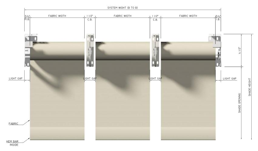
M.B. = MOTOR BRACKET I.B. = IDLE BRACKET
