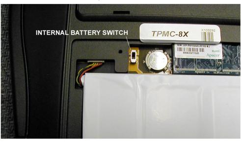
TPMC-8X Internal Battery Switch
