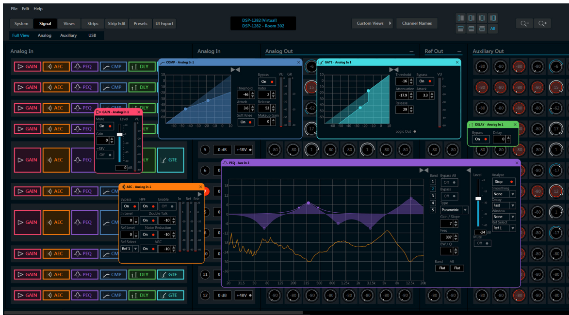
The DSP-128 Tool software workspace with several DSP objects open including a parametric equalizer with spectrum analyzer
