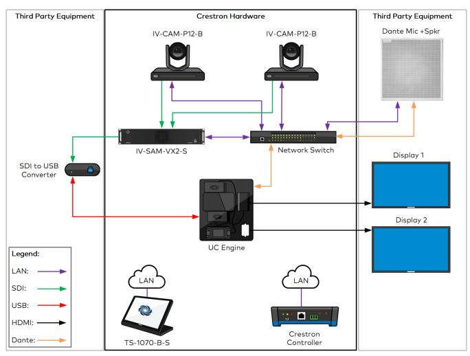
The following diagram provides an example of devices and connections that are common within a typical Automate VX2 deployment.
