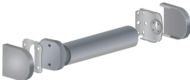
The Crestron Shading Solutions Décor Series utilizes the quiet, precision controlled Quiet Motor Technology (QMT). The Crestron QMT is housed inside the roller shade assembly and controls the movement of the shade, keeps track of the shade's position, and adjusts the shade to the user's desired preset positions.
