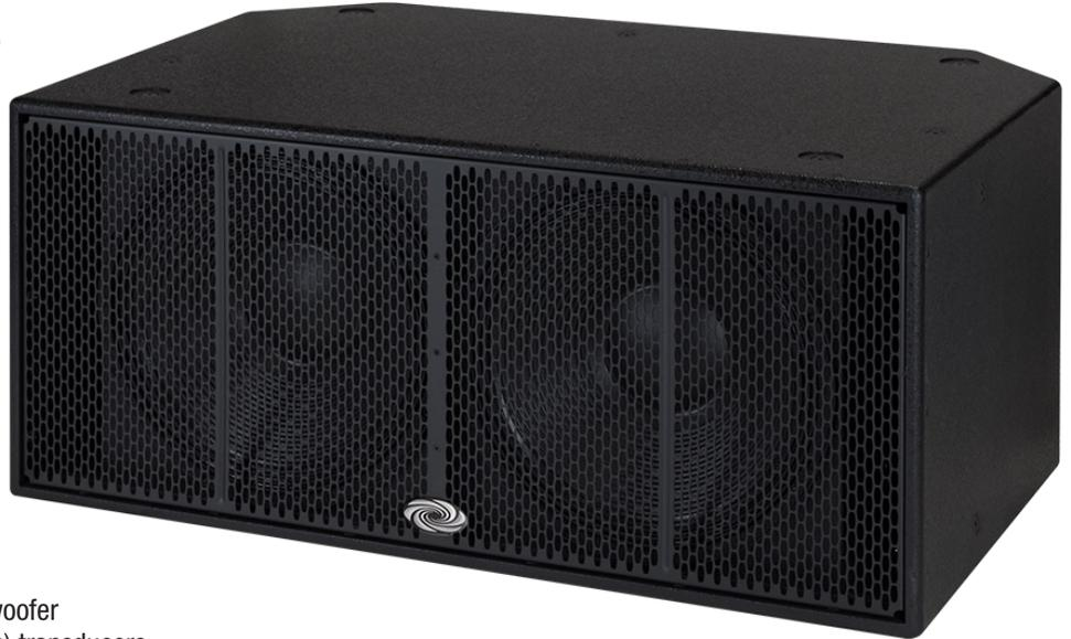
The Vector™ SUBD18 is a direct-radiating, vented subwoofer featuring two high-power, long-excursion 18" (457 mm) transducers. It is designed to provide extended low frequency support for use with CS and CD series Vector Performance Loudspeakers, and is capable of producing articulate and impactful deep bass response for all types of installed music and multimedia applications.
