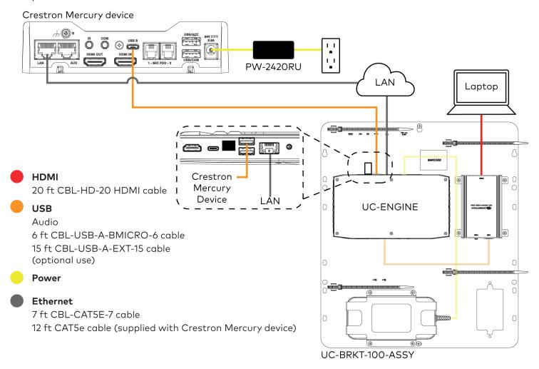
3. Connect the display devices and camera to the UC-ENGINE as shown below.
