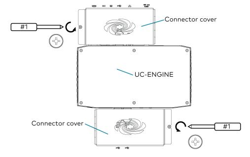
2. Make connections to the Crestron Mercury device and UC-BRKT-100-ASSY bracket assembly as shown in the following illustrations.
