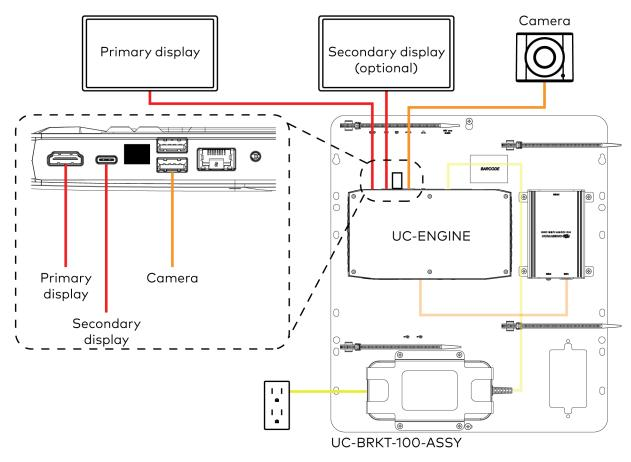
4. Bundle the cables with the integrated cable tie wraps. The cable tie wraps are reusable.
