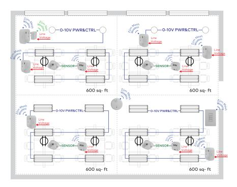
Open offices are controlled separately in zones with floor areas no greater than 600 sq ft. When a zone is vacant for 20 minutes, lights automatically reduce by 80%. If all zones are vacant, the lights turn off. For more information, refer to code section C405.2.1.3.
