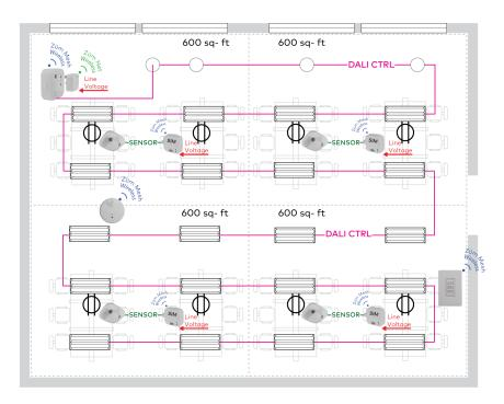
Open offices are controlled separately in zones with floor areas no greater than 600 sq ft. When a zone is vacant for 20 minutes, lights automatically reduce by 80%. If all zones are vacant, the lights turn off. For more information, refer to code section C405.2.1.3.
