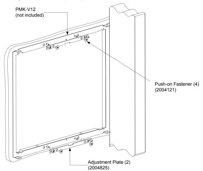
2. Slide a push-on fastener over each pin of the PMK-V12 (or BB-V12) to loosely secure the adjustment plate and the mounting plate. Do not push the push-on fasteners all the way down onto the pins. Slide them on enough to keep the adjustment plate and mounting plate as one adjustment/mounting plate assembly.
