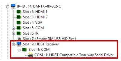
When the third-party HDBaseT receiver device is added to slot 9, the HDBaseT Receiver symbol adds a COM port to the device and enables two-way serial communication.
