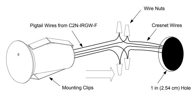
**NOTE:** To ensure proper operation, the C2N-IRGW-F should not be painted.
