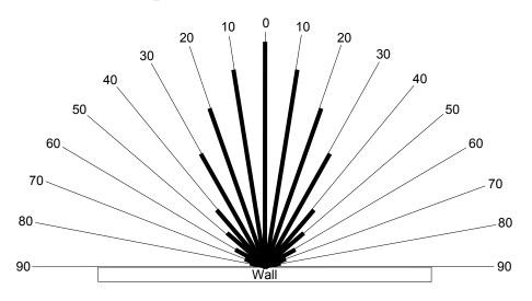
C2N-IRGW-F Vertical Reception Angle (Distance will depend on the remote/transmitter)
