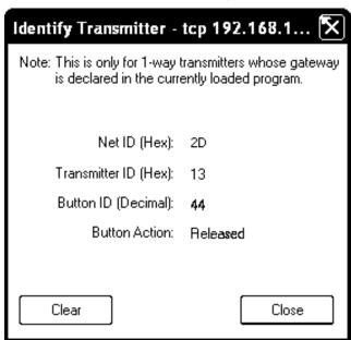
The next logical question is, "What is the *Button ID*?" The purpose of this next procedure is to map the buttons on the universal remote so that a list can be generated and used for reference when creating the SIMPL Windows program. A decimal identification number (or *Button ID (Decimal)* as shown in the "Identify Transmitter" window) corresponds to each physical press on the universal remote. This procedure picks up where the code verification procedure left off.
