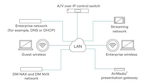
Consideration must be given to blocking at both the switch level and the network design level. DM NAX network switches must have enough switch fabric bandwidth to support full nonblocking bidirectional gigabit bandwidth on all ports simultaneously.
