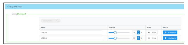
Give each zone a friendly name using the **Name** column of the **Zones** table. If the device is paired with a control system, these names may be overwritten by the control system's program.
