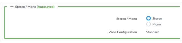
Select either **Stereo** or **Mono**. If **Stereo** is selected, both output channels can have independent audio content. If **Mono** is selected, both output channels receive the same audio content.
