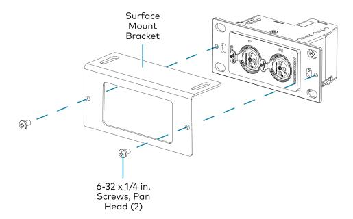
3. Secure the mounting bracket to a flat surface using the appropriate mounting screws (not included).
