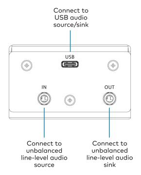
Connect a USB audio source to the **USB** port using a USB Type-C male connector .
