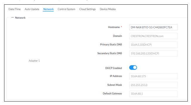
**NOTE:** By default, the hostname of the DM-NAX-BTIO-1G consists of the model name followed by the MAC address of the device. For example, DM-NAX-BTIO-1G-00107FB58088.
