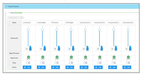
Signal Presence indicates whether or not an audio signal is detected in that zone.
