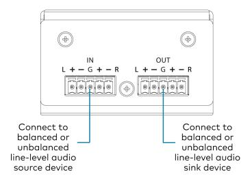
Connect a balanced or unbalanced line-level audio source signal to the INPUTS 5-pin terminal block.
