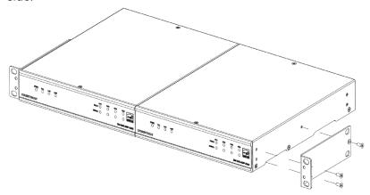
5. Mount the assembly into the rack using four rack mounting screws (not included).
