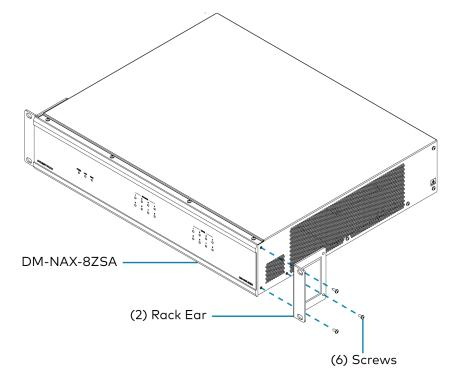
3. Mount the device into the rack using four rack mounting screws (not included).
