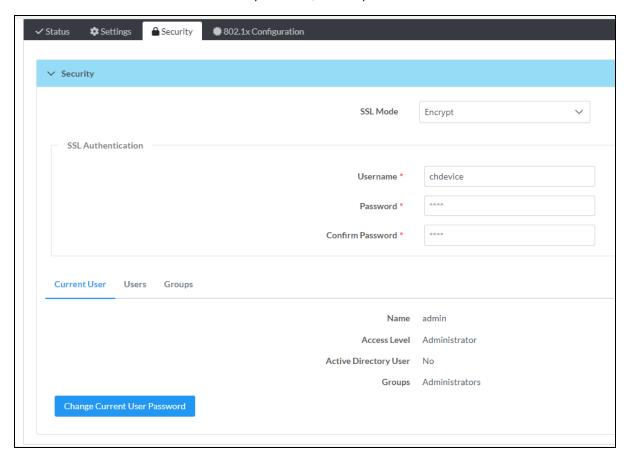
Select **Encrypt and Validate**, **Encrypt**, or **OFF** in the **SSL Mode** drop-down menu, to specify whether to use encryption. By default, SSL Mode is set to **OFF**.
