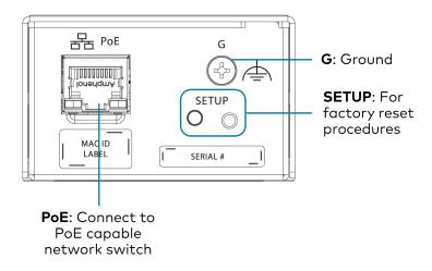
**NOTE: PoE** is a PoE powered device (PD) port. In order for the port to receive PoE, it must be connected to a PoE compliant Ethernet switch.
