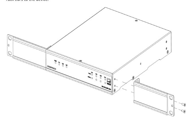
2. Mount the device into the rack using four rack mounting screws (not included).
