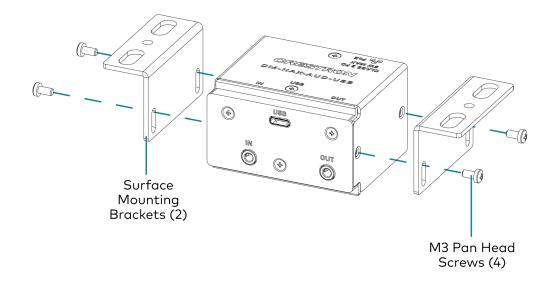
4. Secure the device to a surface or under a table using the appropriate mounting screws (not included).
