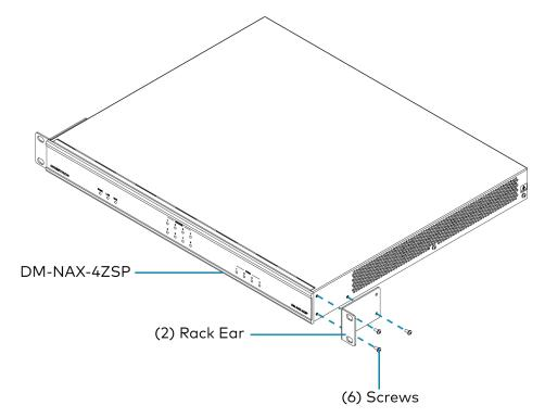
3. Mount the device into the rack using four rack mounting screws (not included).
