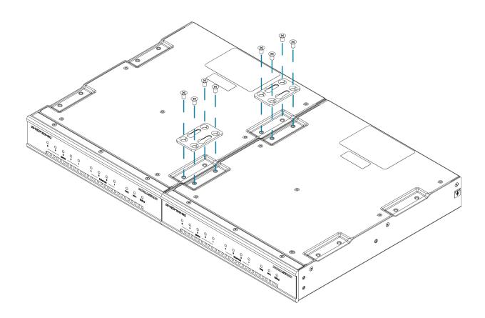
3. Turn the device assembly over and, using six  $6-32 \times 5/16$  in. screws, attach the rack ears to each side.
