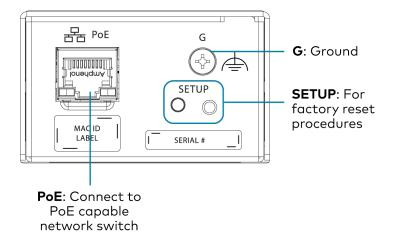
**NOTE: PoE** is a PoE powered device (PD) port. In order for the port to receive PoE, it must be connected to a PoE compliant Ethernet switch.
