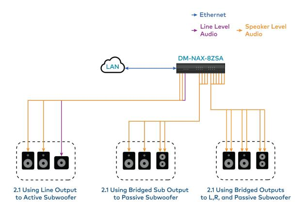
This application diagram shows different 2.1 configurations and how they affect the zone count of an DM-NAX-8ZSA. By default, a zone comprises two speaker outputs (a left and a right).
