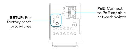
**NOTE: PoE** is a PoE powered device (PD) port. In order for the port to receive PoE, it must be connected to a PoE compliant Ethernet switch.
