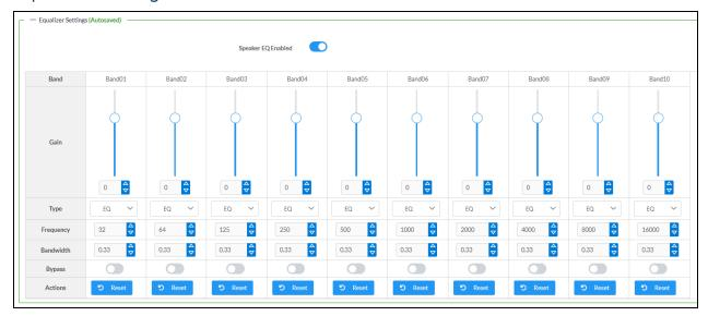
Each output channel of the DM-NAX-AUD-USB has a dedicated ten-band equalizer that can be fully customized to tune the zone output signal to the needs of an install. Each band can have a discrete gain, filter type, center frequency, and bandwidth set, and can also be bypassed. The equalizer itself can also be bypassed using the **Speaker EQ Enabled** toggle.
