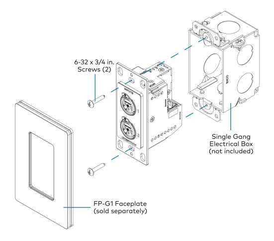
3. Using a Phillips screwdriver and two  $6-32 \times 1/4$  in., flat head screws (not included), attach a FP-G1 decorator style faceplate (sold separately) to the wall plate.
