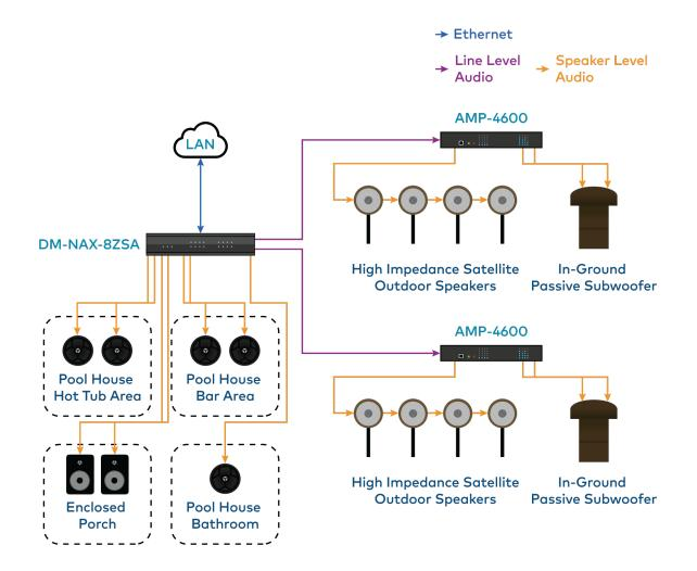
This application diagram shows zones using only the line outputs. Line outputs 1 and 2 feed high impedance amplifiers driving speakers for large outdoor spaces and speaker zone outputs 5-8 feed low-impedance indoor spaces without overlap of signals. The LAN cloud shows that any individual applications can exist as part of a large DM NAX system.
