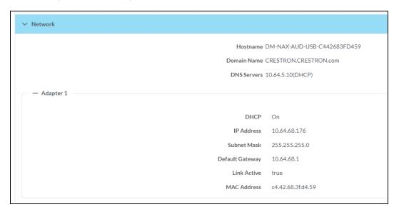
**NOTE:** By default, the host name of the DM-NAX-AUD-USB consists of the model name followed by the MAC address of the device. For example, DM-NAX-AUD-USB-00107FB58088.
