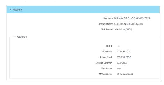
**NOTE:** By default, the host name of the DM-NAX-BTIO-1G consists of the model name followed by the MAC address of the device. For example, DM-NAX-BTIO-1G-00107FB58088.
