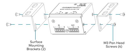
4. Secure the device to a surface or under a table using the appropriate mounting screws (not included).
