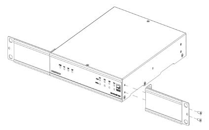
3. Mount the device into the rack using four rack mounting screws (not included).
