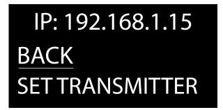
After selecting **SET TRANSMITTER**, a status page is briefly displayed indicating that the device is switching to transmitter mode, followed by the temporary **STARTING UP** page.
