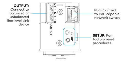
**NOTE: PoE** is a PoE powered device (PD) port. In order for the port to receive PoE, it must be connected to a PoE compliant Ethernet switch.
