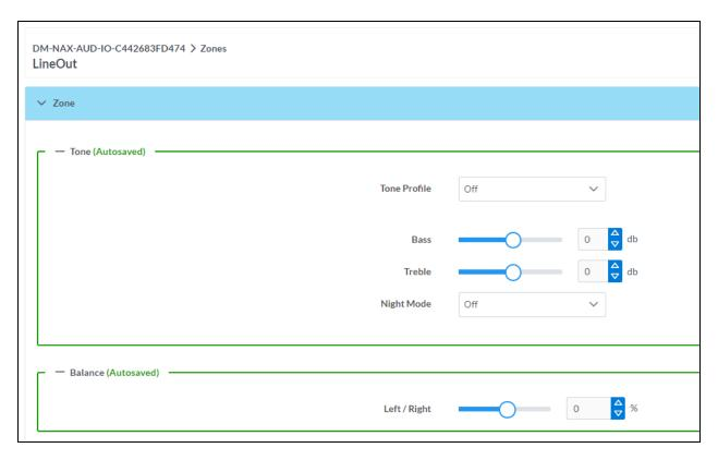
The **Tone** section provides adjustments for the **Tone Profile**, **Bass**, **Treble**, **Loudness**, and **Night Mode** settings of the zone output.
