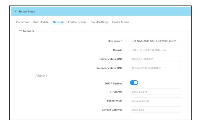
**NOTE:** By default, the host name of the DM-NAX-AUD-USB consists of the model name followed by the MAC address of the device. For example, DM-NAX-AUD-USB-00107FB58088.
