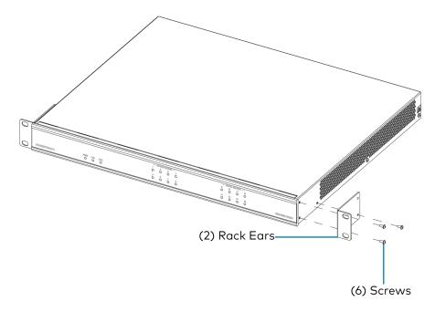
3. Mount the device into the rack using four rack mounting screws (not included).
