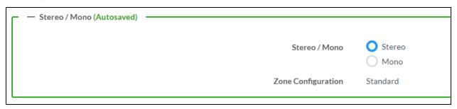
Select either **Stereo** or **Mono**. If **Stereo** is selected, both output channels can have independent audio content. If **Mono** is selected, both output channels receive the same audio content.
