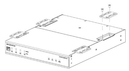
2. Position the device as desired and use screws (not included) and anchors (not included) to mount it.
