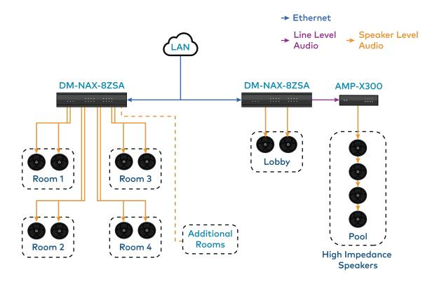
This application diagram shows a commercial setup using casting service streaming applications. For example, in a hotel, each room can receive a cast from a third-party device. The Lobby and Pool zones can exist on another DM-NAX-8ZSA unit that is on the same LAN or on a separate VLAN or WAP to cast to/control those zones.
