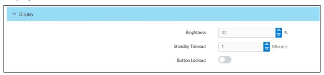
The **Display** section contains settings that affect the front panel OLED display of the DM-NAX-BTIO-1G.
