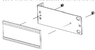
4. Turn the amplifier assembly over and, using  $\sin 6-32 \times 3/8$  in. screws, attach the rack ears to each side.
