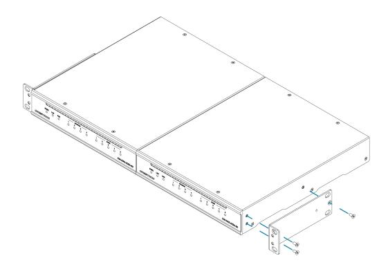
4. Mount the assembly into the rack using four rack mounting screws (not included).
