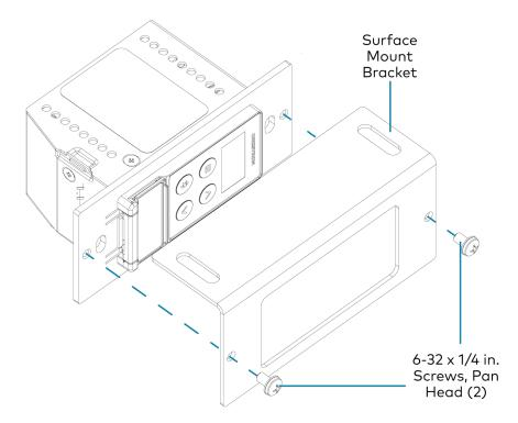
3. Secure the device to the underside of a table using the appropriate mounting screws (not included).
