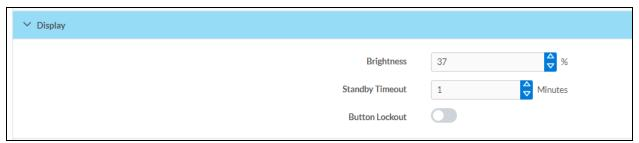
The Display section contains settings that affect the front panel OLED display of the DM-NAX-BTIO-1G.
