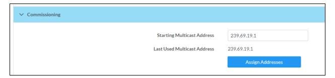
Select **Assign Addresses** to give each DM NAX transmitter in the DM-NAX-AUD-USB a unique multicast address beginning with the specified **Starting Multicast Address**. The valid range for **Starting Multicast Address** is 239.8.0.0 to 239.127.255.254.
