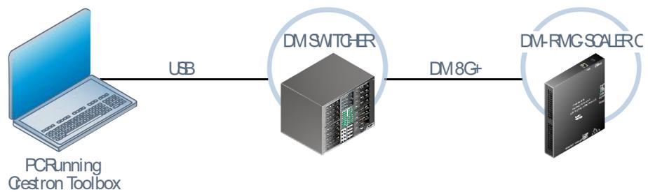
To establish USB communication between the PC and the DM-RMC-SCALER-C via a DM switcher:
