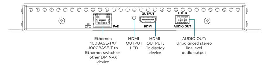
DM-NVX-E10 and DM-NVX-D10 Rear Panel Connections
