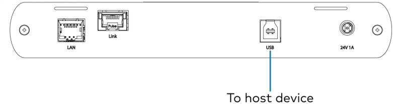
3. Connect each USB extender to its included power adapter, then connect each power adapter to an AC power source.
