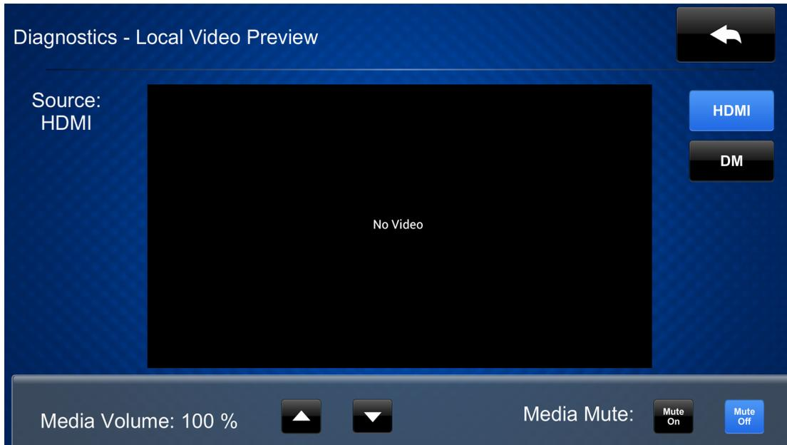
Use the **Diagnostics - Local Video Preview** screen to preview the video source that is connected to either the HDMI input or DM<sup>®</sup> input.
