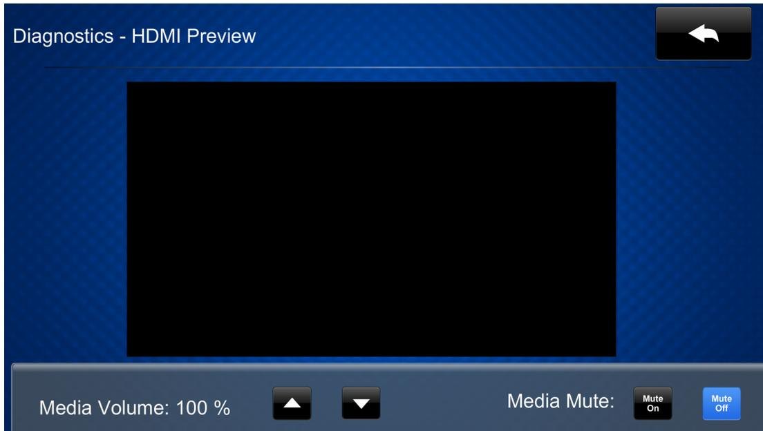
Use the **Diagnostics - HDMI Preview** screen to preview the video source that is connected to the HDMI® input.
