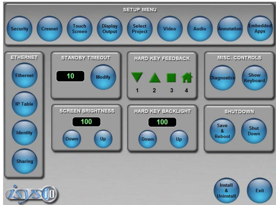
The SETUP MENU provides access to all basic functions and parameters. It is divided into *SETUP*, *ETHERNET*, *STANDBY TIMEOUT*, *HARD KEY FEEDBACK*, *MISC. CONTROLS*, *SCREEN BRIGHTNESS*, *HARD KEY BACKLIGHT* and *SHUTDOWN* sections. An **Install & Uninstall** button is also provided for adding third-party software applications like Skype™ and for installing wireless network cards.
