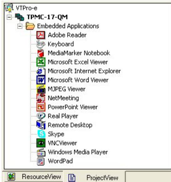
Right-click on any of the applications in the *Project View* and select **Properties** to open the “Embedded Application Property” window (refer to illustration on the following page). This window permits a choice of positions on the screen, assignment of an analog touch join type and number and a show/hide join number.
