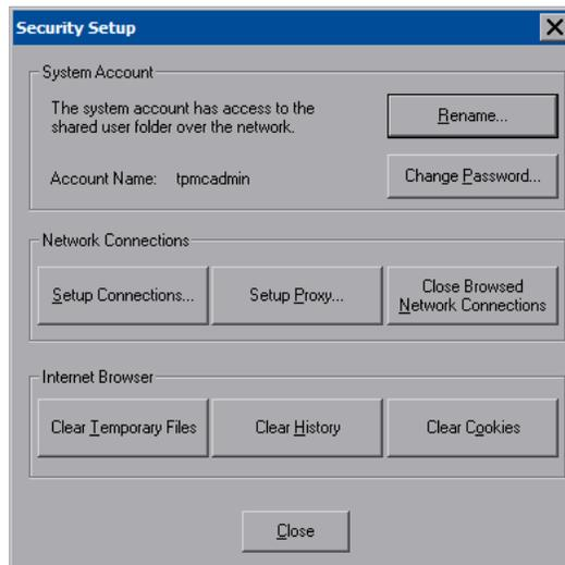
Click **Setup Connections...** to open the “Network Connections” window. This window is used to map to a network drive. A mapped network drive permits easy access to embedded application files (Word, Excel, PowerPoint, MediaMarker, etc.) and provides a location to save files. To further customize the installation, network drives containing compiled touchpanel project files can also be mapped.
