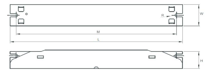
L: 16.7 in (425 mm) M: 16.1 in (408 mm) W: 1.2 in (30 mm) H: 0.8 in (21 mm) R: 0.05 in (1.3 mm)
