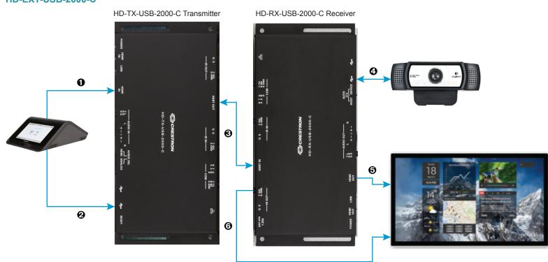
The HD-EXT-USB-2000-C consists of two components: the HD-TX-USB-2000-C transmitter and the HD-RX-USB-2000-C receiver.
