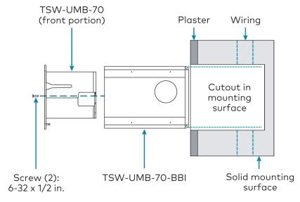
The TSW-UMB-70-BBI can also be mounted vertically for use with the TSW-570P portrait touch screen.
