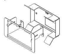
Only the front portion of the TSW-UMB-70 is required for installation with the TSW-UMB-70-BBI. The rear portion may be discarded or retained for future use.
