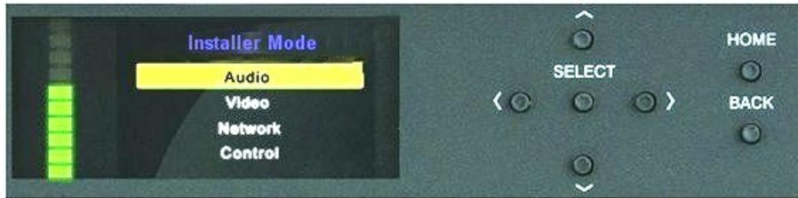
Use the buttons adjacent to the left, right, up, and down arrow symbols on the front panel to navigate the various menus and options. The **SELECT** button accepts the displayed menu option or value; the **HOME** button returns the display to the initial display; the **BACK** button always returns the display to the previous screen. There are four options within the “Installer Mode” menu.
