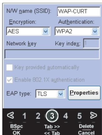
In the screens opened by the **WiFi Access Point**, **CntlSystem IP Address** and **IP Config** buttons, a keyboard application is displayed at the bottom. The keyboard uses the navigation pad (up, down, left and right) to select a character to type. The center button on the navigation pad types the selected character.
