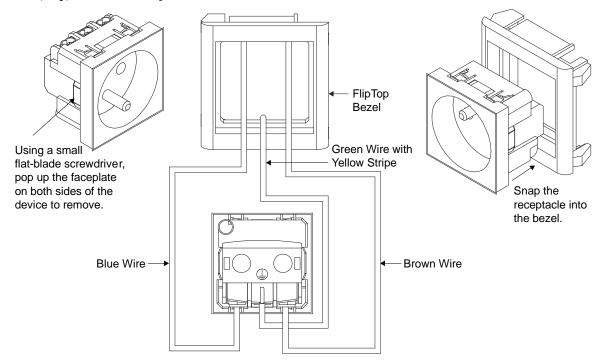
After the faceplate has been removed, loosen the appropriate screws, insert the wires as shown in the illustration above, and tighten the screws using a small flat-blade screwdriver. Replace the faceplate, orient the receptacle as shown, and snap the receptacle into the bezel.
