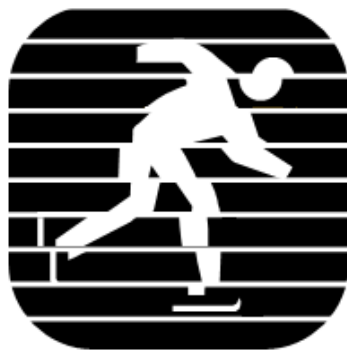
Motion Alternate Line Displacement in Interlaced Scan
