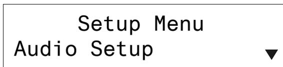
Press the **ENTER** button to select which parameter of the Audio Setup menu you wish to view. From any of the parameter level menus, you can select a different parameter by using the rotary quick-adjust knob on the front panel.
