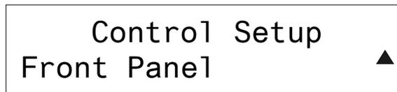
To turn the front panel lock on or off, press **ENTER**. Use the quick-adjust knob to set the front panel lock on or off.
