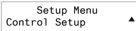
Press the **ENTER** button to select which parameter of the Control Setup menu you wish to view. From any of the parameter level menus, you can select a different parameter by using the rotary quick-adjust knob on the front panel.
