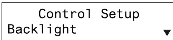
To set the backlight level, press **ENTER**. Use the quick-adjust knob to set the backlight level to Low, Medium or High.
