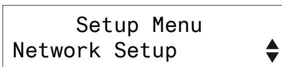
Press the **ENTER** button to select which parameter of the Network Setup menu you wish to view. From any of the parameter level menus, you can select a different parameter by using the rotary quick-adjust knob on the front panel.
