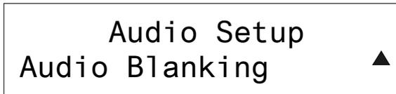
To set audio blanking, press **ENTER**. Use the quick-adjust knob to turn audio blanking on or off.
