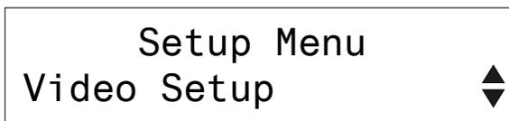
Press the **ENTER** button to select which parameter of the Video Setup menu you wish to view. From any of the parameter level menus, you can select a different parameter by using the rotary quick-adjust knob on the front panel.
