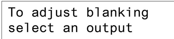
Press the front panel **OUT** button for the output you wish to adjust.
