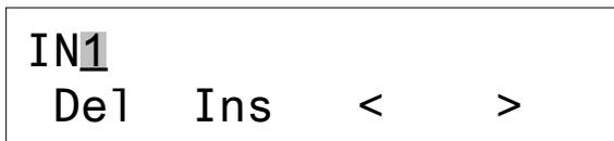
Use the buttons below the < and > symbols on the display to navigate to the digit you wish to set. Use the buttons below **Del** and **Ins** to delete and/or insert digits. Change a digit by rotating the quick-adjust knob.
