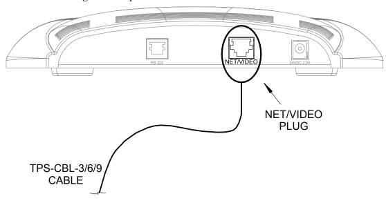
2. Refer to the diagram below. At the TPS-4500IMC (or optional TPS-4500IMW, not shown), attach the cable plug labeled **NET/VIDEO** to the **NET/VIDEO** port.
