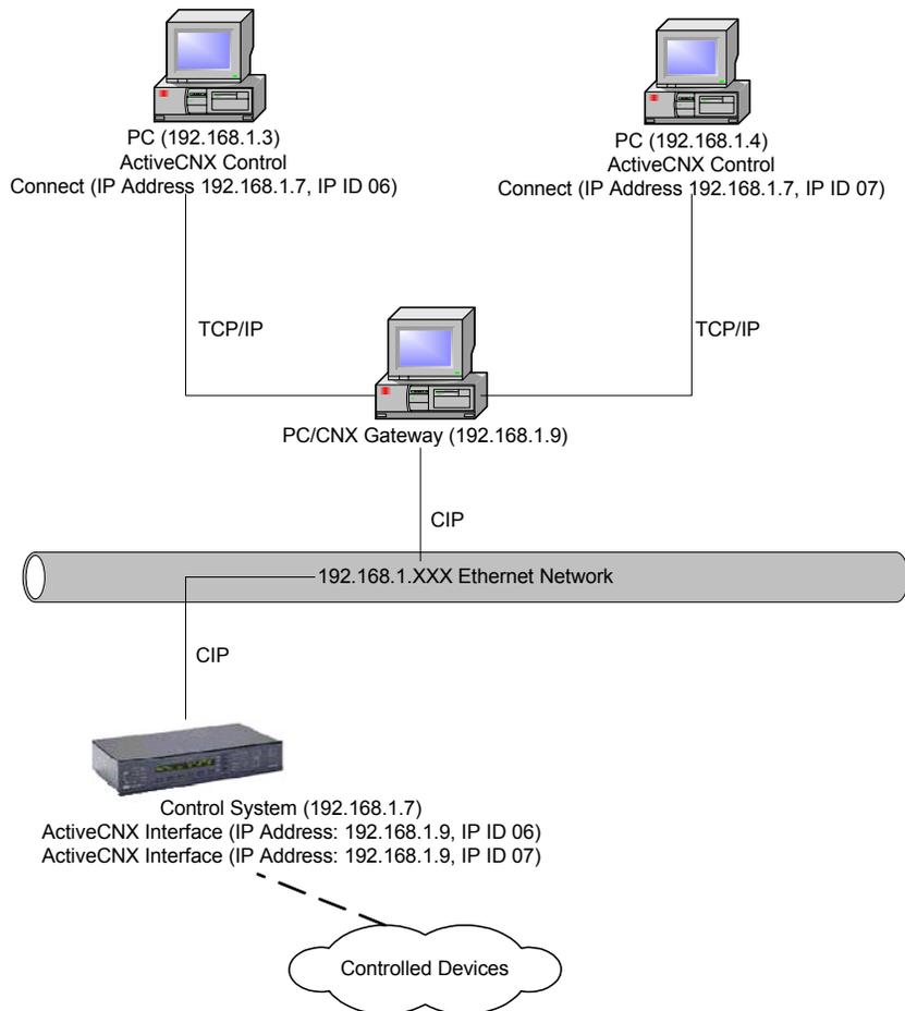
The ActiveCNX control can also communicate directly with a CEN device. In this configuration, the CNX-EGWY is required, since the CEN device does not provide an internal “hardware” gateway.
