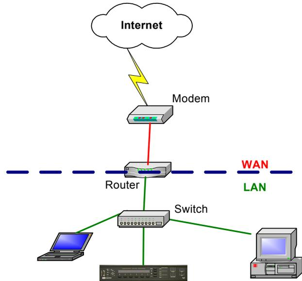
The router’s firewall (NAT, or Network Address Translator) protects the internal LAN by inspecting the data coming in from the WAN port before delivery to the final destination on the LAN port. The router inspects Internet port services like the Web server, FTP server, or other Internet applications, and, if allowed, it will forward the data to the appropriate PC or control system on the LAN side.
