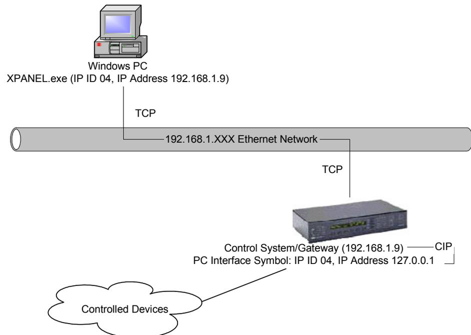
Two gateway configurations enable a Web browser to access the control system. In both cases, the e-Control gateway must reside on the same machine as the Web server containing the HTML pages. This applies to both Java-based and e-Control 2 pages.
