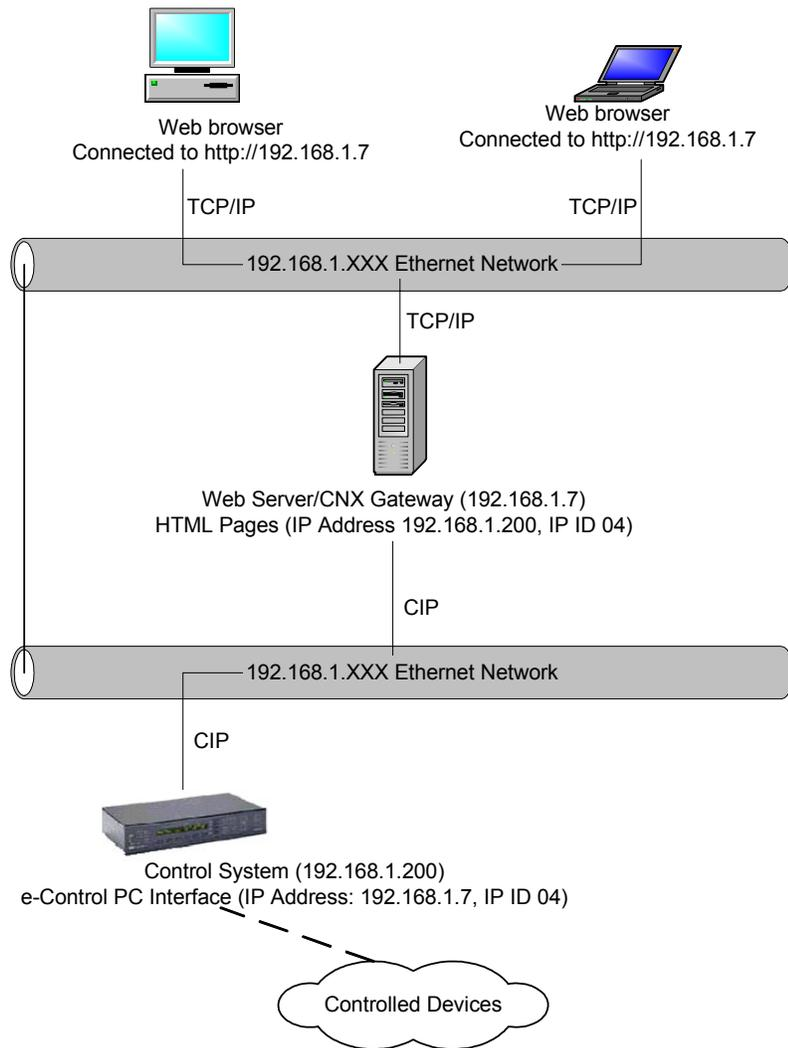
The configuration shown below uses the “hardware” gateway that is built into the 2-Series control processor; the Web pages are stored in the control system’s internal Web server. This configuration supports a maximum of 30 simultaneous connections. (The CNXENET+ card supports up to five simultaneous connections.)
