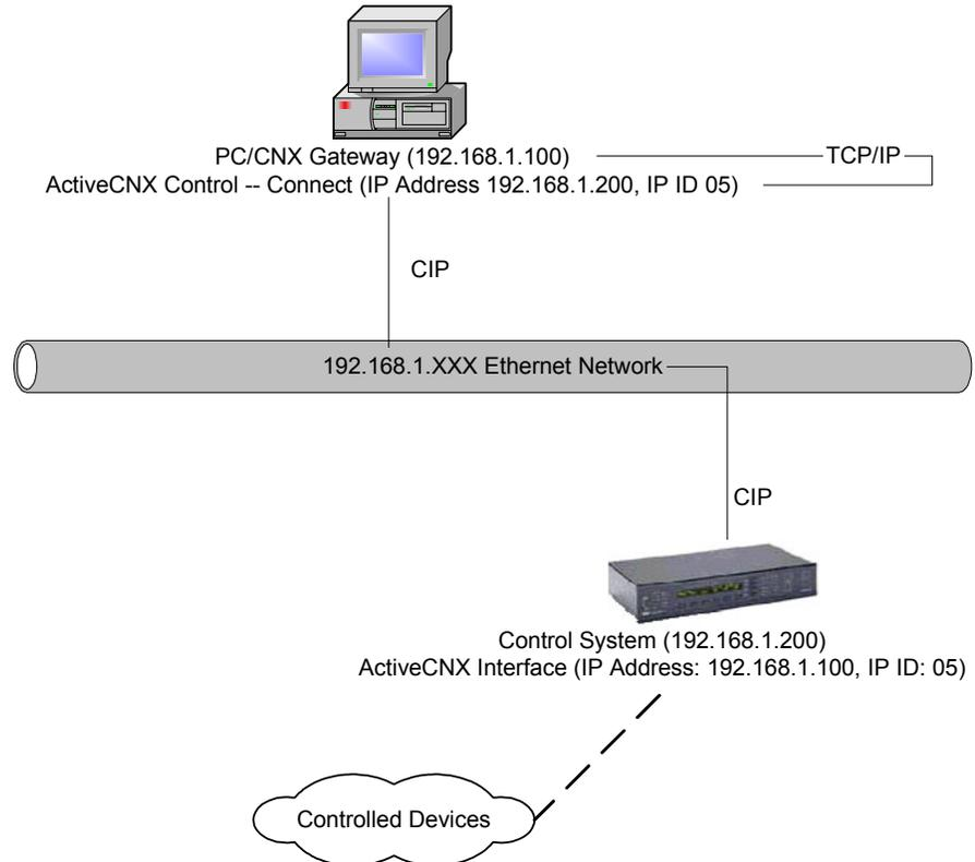
Once a connection is established, data can pass back and forth between the PC application and the control system, just as with any other interface. As commands are sent to the control system, the control system forwards the commands to controlled devices. Feedback from the devices is sent to the control system and goes back in real time to the PC application.
