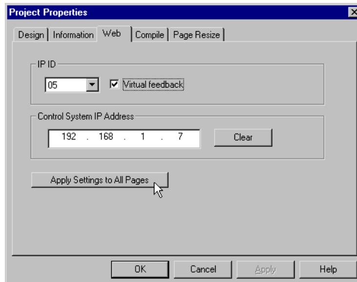
As shown in the previous diagram, you can click **Apply Settings to All Pages** to set the same IP information to all the pages in the browser project. You can also click the **Virtual feedback** check box if you want to enable “instant” feedback. This feature causes an object such as a button to display in its active state the moment the user clicks it, even if there is some delay in receiving actual feedback from the controlled device.
