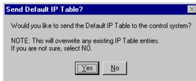
The second method for creating the IP Table enables you to set or change the IP information and send it to the control system without need to re-compile or re-transfer the SIMPL Windows program.
