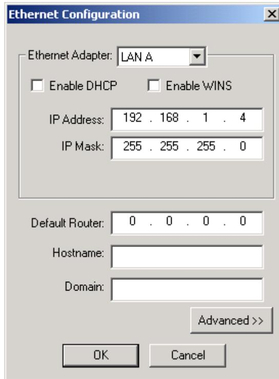
4. Static IP values can be set for the LAN B side of the C2ENET-2 card the same way. Simply select **LAN B** from the **Ethernet Adapter** list.
