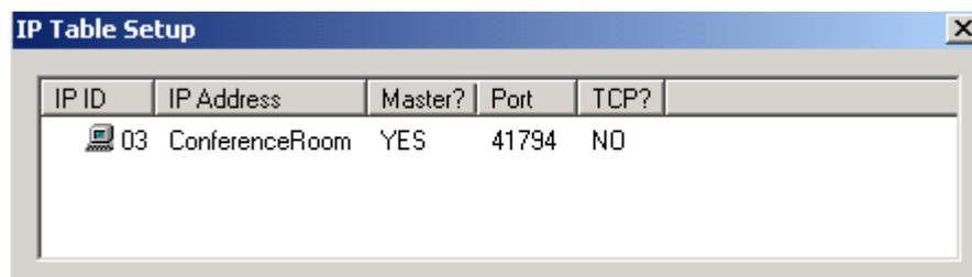
2-Series control systems operating in slave mode can accept commands only from one control system; thus, the IP Table (Master List) will consist of only one entry.
