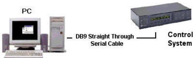
2. Start the Crestron Viewport and click **Communication Settings** on the **Setup** menu. Select **RS-232** as the connection type. Then set the PC to match the communication settings of the control system:
