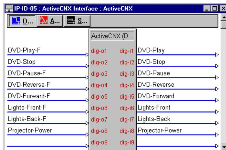
The Active CNX control initiates a connection to the control system—and its associated ActiveCNX Interface symbol—through a method, or internal command, called Connect( ). This method has two parameters: 1) The IP address or fully-qualified domain name of the control system; and 2) The IP ID of the ActiveCNX Interface symbol, as set in SIMPL Windows.
