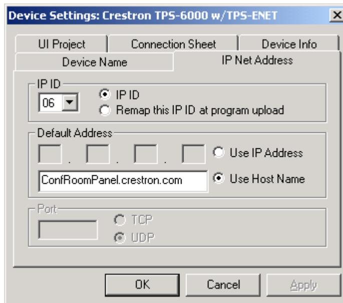
5. **For Generic Ethernet Modules:** The device settings for Generic Ethernet modules such as the ActiveCNX Interface and e-Control PC Interface are the same regardless of the DHCP setting.
