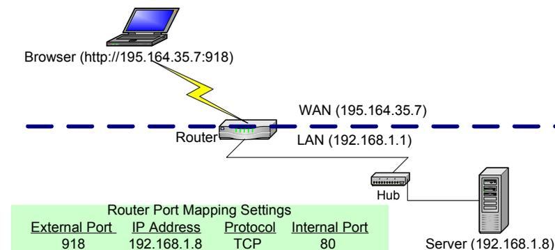
Most routers allow between 10 and 16 ports to be opened using port mapping; the Crestron NAT that is built into the 2-Series processor allows up to 16.
