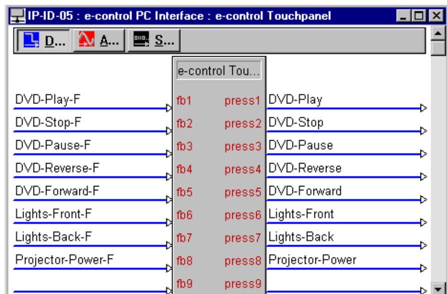
Once the Web browser establishes a TCP/IP connection to the e-Control gateway, data can pass back and forth between the browser and the control system, just as with any other interface. The gateway receives commands from the browser over TCP, performs the translation to CIP and forwards the data to the control system. Feedback from the control system is routed back by the gateway to the Web browser.
