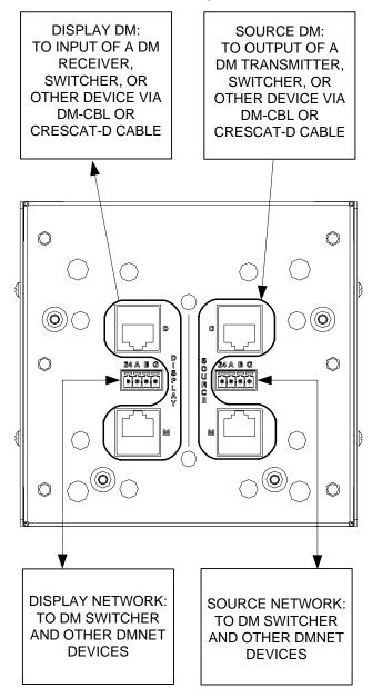
**NOTE:** Ensure the unit is properly grounded.
