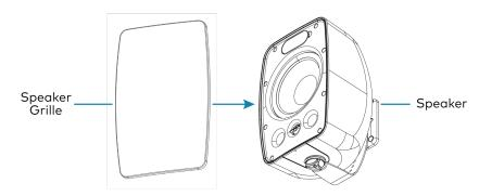
6. Fasten the grille to the top and bottom of the speaker housing using the two security screws removed during step 5a.
