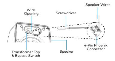
c. When wiring multiple speakers in parallel (70V or 100V run), connect the OUT + and - terminals to the subsequent speaker's IN + and - terminals. Preserve proper polarity by connecting OUT + to IN + and OUT - to IN -.
