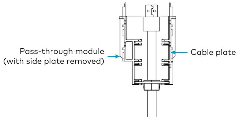
3. Attach the side plate to the module by snapping the plastic clips on the plate into the two slots on the module.
