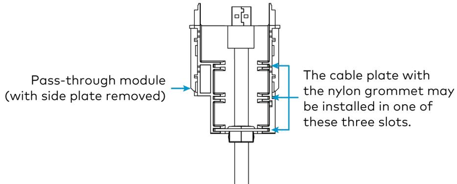
6. Attach the side plate to the module by snapping the plastic clips on the plate into the two slots on the module.
