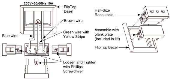
After connecting the wires as shown in the illustration, orient the receptacle as shown and snap the receptacle into the bezel using the supplied blank plate.
