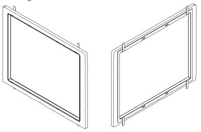
**NOTE:** The mounting plate will have slight play; this is normal. It allows for minor adjustments to the touchpanel during installation.
