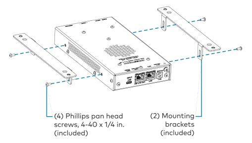
Bracket Attachment for HD-TXU-4KZ-211 and HD-TXU-4KZ-211-CHGR Under Table Mounting (HD-TXU-4KZ-211-CHGR Shown)
