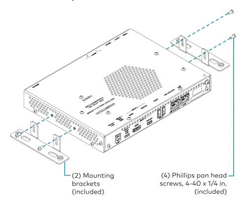
Bracket Attachment for HD-RXU-4KZ-202 Wall Mounting
