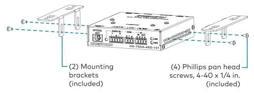
Bracket Attachment for HD-TX-4KZ-201/401/211-CHGR/421-CHGR Under Table Mounting (HD-TX-4KZ-421-CHGR Shown)
