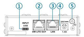
USB INPUT Port: USB Type-C® connector, female; Digital video/audio input using DisplayPort Alt Mode (CBL-USB3G1-C-C-6 and CBL-USB3G2-C-C-3 cables sold separately); USB 2.0 data support
