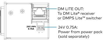
Connections to Rear of HD-RX(C)-4KZ-101-1G Series Receiver
