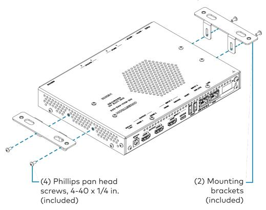
2. Using four screws (not included), attach the device to the underside of a table. For example purposes, the HD-TXCA-4KZ-101 is shown in the following illustration.
