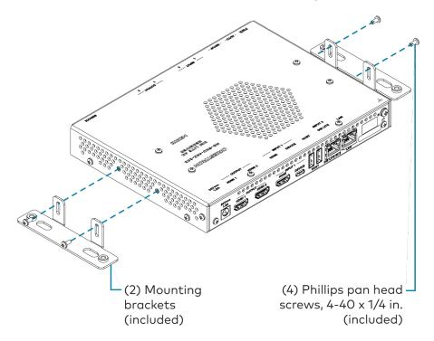
2. Using the four included anchors, washers, and  $6-32 \times 3/4$  in. combo truss head screws, attach the device to the wall. For example purposes, the HD-TXCA-4KZ-101 is shown in the following illustration.
