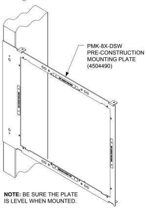
CAUTION: Allow an air gap of at least 12 inches (30.48 cm) in the wall cavity above and below the TPMC-8X-DSW for heat dissipation.
