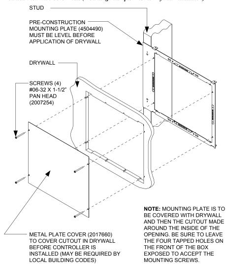
Mounted View with Cover Plate (Mounting Example Prior to Drywall Installation)
