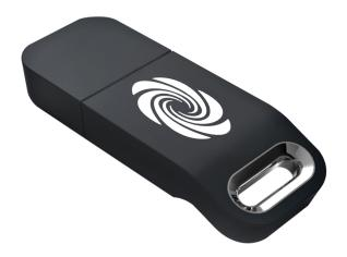
The Crestron® <u>USB-OFFLINE</u> is a USB dongle that provides a means for validating Crestron Virtual Control (VC-4) room licenses and BACnet licenses offline without requiring an XiO Cloud® service account. The USB-OFFLINE is ideal for Crestron Virtual Control installations that require offline licensing. The USB-OFFLINE is compatible with the <u>VC-4-PC-3</u> Dell® micro computer or a standalone <u>VC-4 server</u>.
