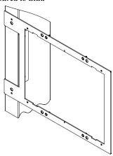
The plate is designed to provide the necessary support for a single touchpanel and can mount to the right or left side of a stud. Confirm that the PMK-3100L is level before application of drywall. A rectangular opening with the dimensions shown in the illustration after this paragraph must be made in the drywall. Verify that the opening exposes the #6-32 tapped holes in each corner.
