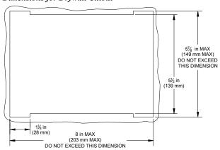
If the opening for the touchpanel in the drywall is too large, two pre-construction accessories are available to make adjustments. Use the optional TMK-3100L (Trim Ring Kit) to provide a smooth edge at the opening. This option provides a finished appearance and is preferred when wallpaper is hung. Use the optional MMK-3100L (Mud Ring Kit) to fill in larger irregularities around the opening (requires plastering).
