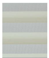
Puckered, dimpled or pinched fabrics are caused by the shrinkage or stretching of one layer among multiple layers of fabric.
