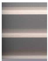
Worm tracks may appear as a slight crease that travels horizontally near the front of the vane, typically seen on the face sheer and in light-dimming fabrics.
