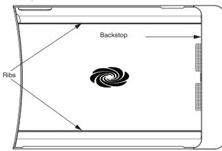
2. Clean the surfaces of the cradle's ribs using the supplied alcohol wipe. Make sure the surfaces are fully dried before continuing to the next step.
